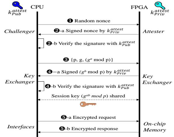
**Figure 4: Secure channel establishment between CPU and FPGA** application, TRUSTLIB asks the device driver to map TRUSTMOD’s memory to TRUSTLIB’s non-EPC memory region which can directly be accessed without an enclave exit.
