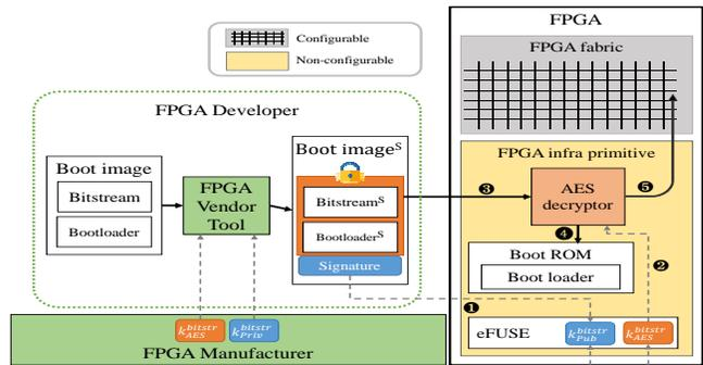
Figure 1: A generic secure boot architecture of FPGA
