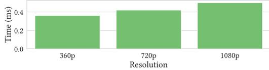
Figure 12: The time taken to prepare a depth map (per frame) while varying its resolution
