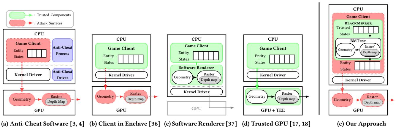
Figure 5: Comparisons between Our Approach, Anti-Cheat Software and Alternative Approaches Using Trusted Execution
