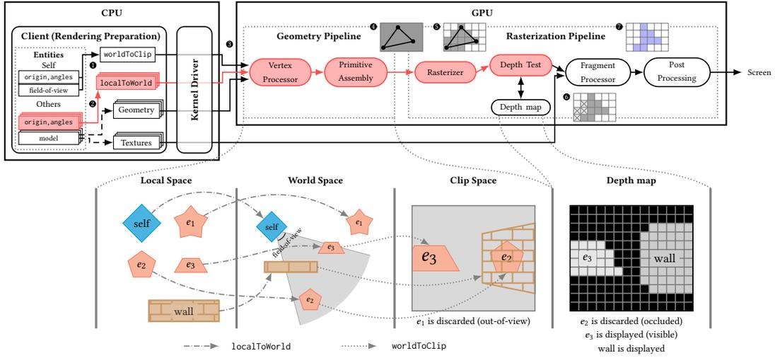
Figure 3: Overview of rendering pipeline (top) and corresponding transformations in coordinate systems (bottom)
