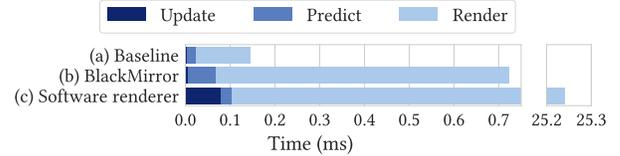
Figure 14: A comparison of the overhead to run a frame. (a) Baseline runs updates and predictions without an enclave, and renders the scene on the GPU. (b) BLACKMIRROR runs updates and predictions within the enclave, and performs trusted visibility testing before rendering the scene on the GPU. (c) Software renderer is identical to the baseline, except that it renders the scene with a software renderer.
