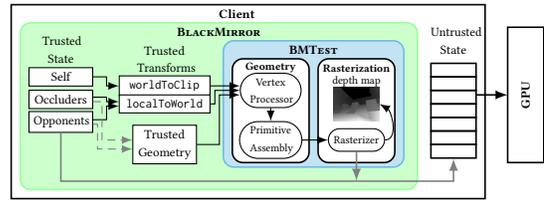
Figure 9: The workflow of BLACKMIRROR’s visibility testing
